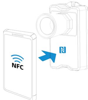
4. Basic information and settings of devices will be shown on ToolBox if it's recognized successfully. You can switch on/off, read and write the device by tapping the button on the Apps. In order to protect the security of devices, password validation is required when configuring via unused phone. Default password is **123456**.
