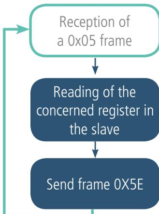
If the request is false or there is an error during reading, this frame will be empty.
